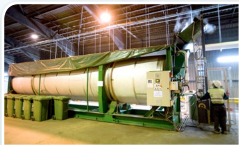
In-vessel composting unit in Kowloon Bay Pilot Composting Plant can handle 2-4 tonnes of biodegradable waste daily. 九龙湾厨余试验处理设施的密封式堆肥装置每日可处理二至四吨生物可降解废物。
