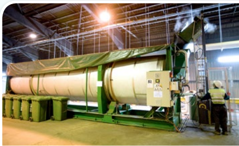
In-vessel composting unit in Kowloon Bay Pilot Composting Plant can handle 2-4 tonnes of biodegradable waste daily. 九龍灣廚餘試驗處理設施的密封式堆肥裝置每日可處理二至四噸生物可降解廢物。
